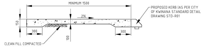
**CONCRETE PATH TYPICAL SECTION – TYPE 2**
