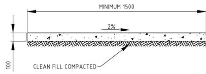
**CONCRETE PATH TYPICAL SECTION – TYPE 1**
