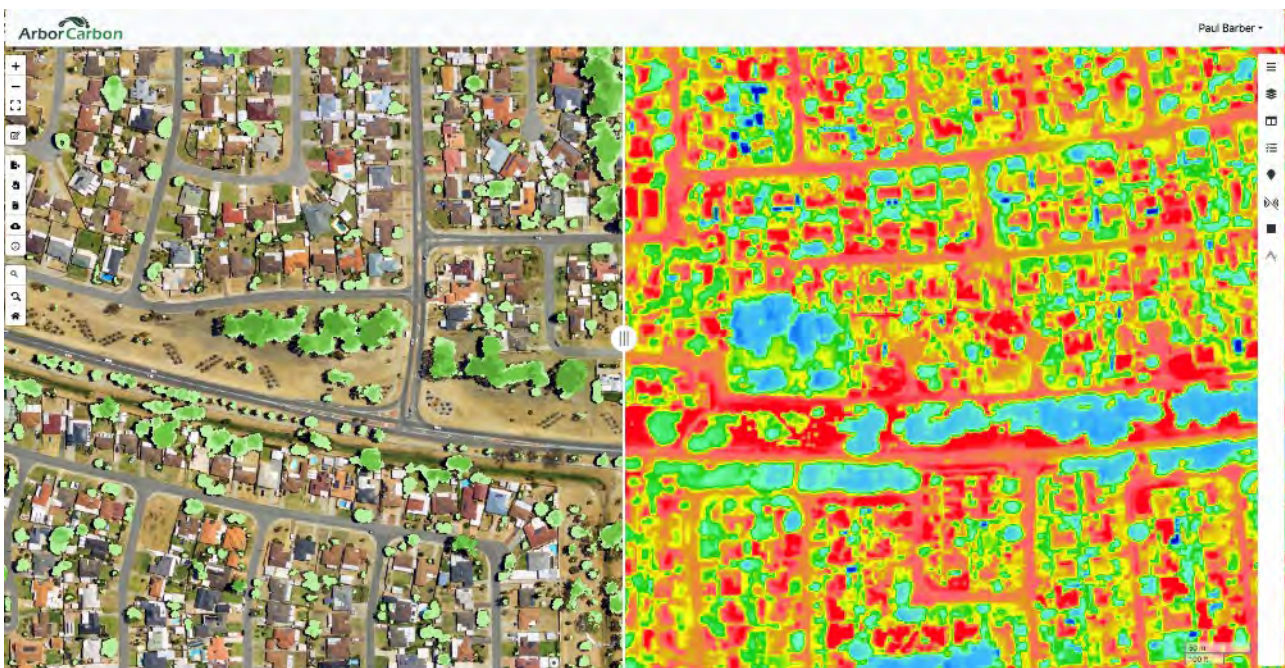
Figure 36: Airborne ArborCam image viewed through a web-portal showing canopy cover (green polygons) overlaid onto a baseline true colour orthomosaic (left), and surface temperatures colour-scaled from cooler temperatures (blue) through to hotter temperatures (red), with trees clearly demonstrating a strong cooling effect).
