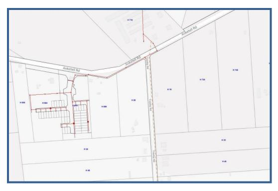
Figure 2 – Existing gravity sewer infrastructure (source: Water Corporation November 2018)
