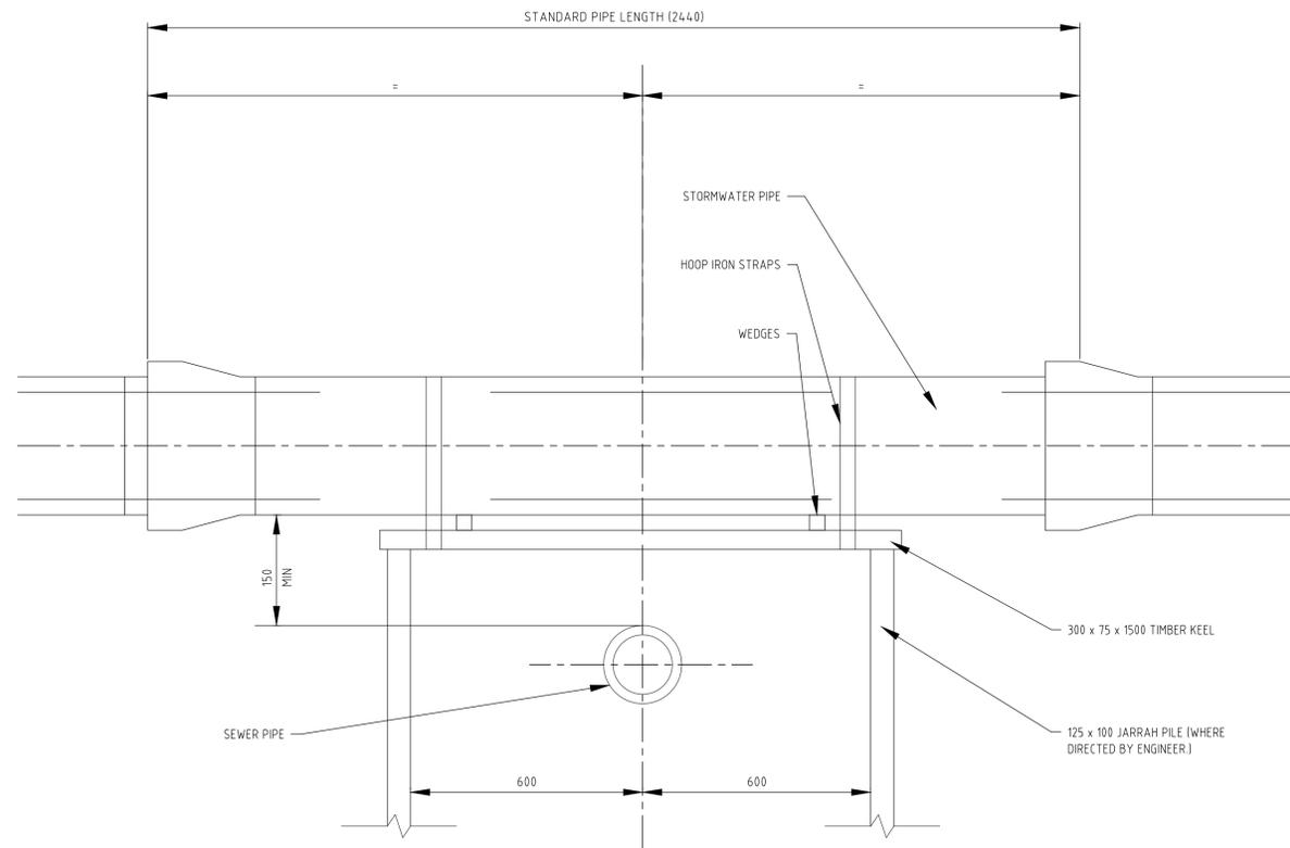
TYPICAL STORMWATER – SEWER CROSSING
