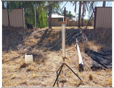
Photo 6. Test Location 02 (FPT2), Conducting Field Permeability Test
