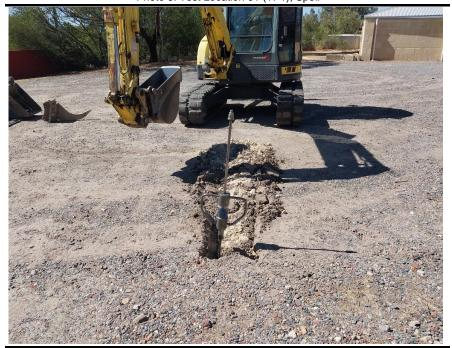
Photo 4. Test Location 01 (DCP1), Testing by using a Dynamic Cone Penetrometer
