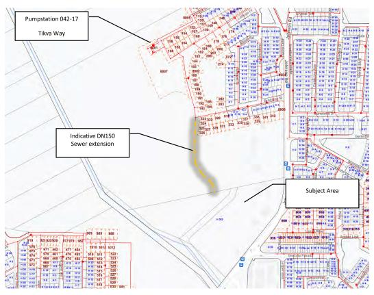
Figure 4: Preliminary Sewer Layout (Esinet)
