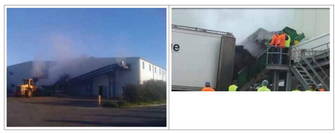
Figure 4 Comparison of hopper loading from front-end loader 25/7/2012 0817 hours and walking floor truck 1/7/2015 0900 hours
