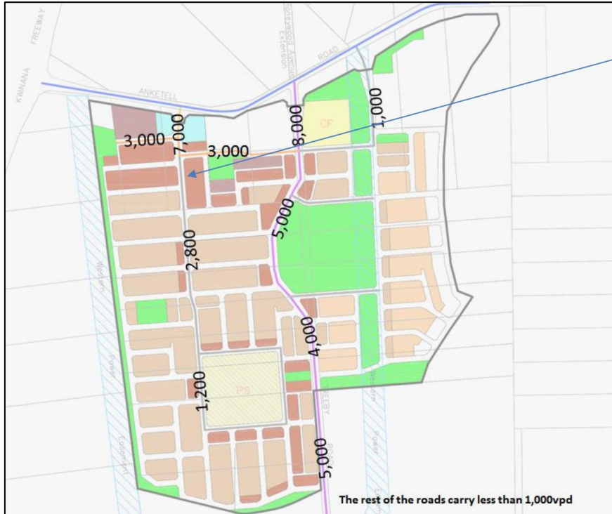
Figure 5: Projected Daily Traffic Volumes (Right-In assumed to be approved at LSP Road 1)
