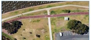
Figure 10: In areas of high pedestrian activity it is critical to provide separation between cyclists and pedestrians
