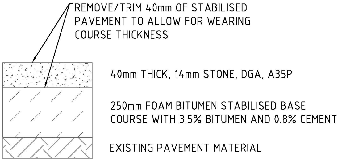
FINISHED PAVEMENT DETAIL
