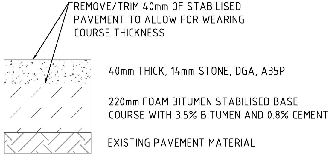
FINISHED PAVEMENT DETAIL
