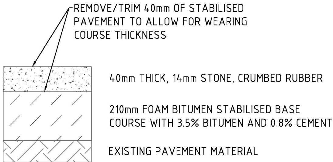
FINISHED PAVEMENT DETAIL
